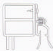
Typical softwall attachment with Simplex Hook Bead mounting bar.
