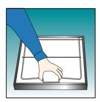
Changing air filter pads are a snap. Simply open the hinged gate, remove the dirty pad and install the clean replacement. The hinged gate design provides superior media support without restricting air flow.
